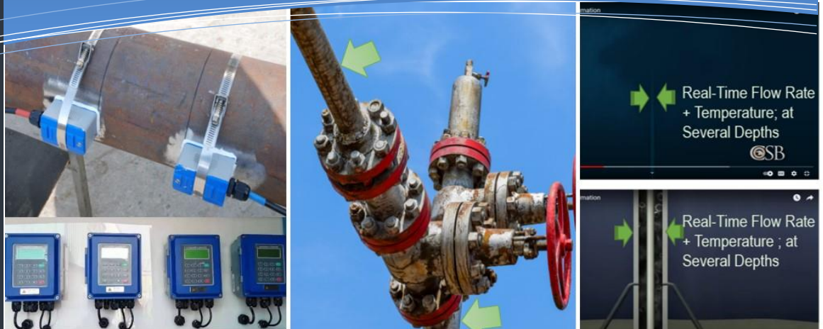
Non-Intrusive Monitoring of Changes in Relative Flow Rate; Flow Path, Present-Absent of Flow Along with Vibration and Temperature Data are Used in Leakage, Operational Errors Alerts
